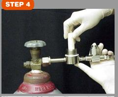
Place new  $LCO_2$  Filter Element (#8784A) into lower Oil/Water Filter Housing. Let gravity hold element in place.
