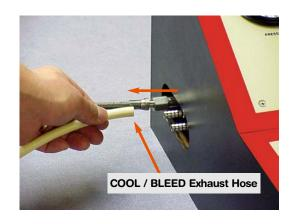
4. Close main LCO<sub>2</sub> tank valve, bleed LCO<sub>2</sub> High Pressure Hose. Disconnect 'LCO<sub>2</sub> High Pressure Hose' using supplied 9/16" Wrench and 1/2" Wrench from the SAMDRI<sup>®</sup>-PVT-3D Connect Inlet.
