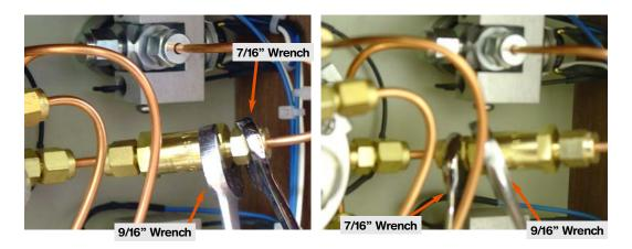
4. Install new Purge Line Filter paying attention to flow direction. Please note flow direction on the Purge Valve MUST be installed in-line with flow direction indicated in previous SAMDRI<sup>®</sup>-PVT-3D Chamber Plumbing picture.
