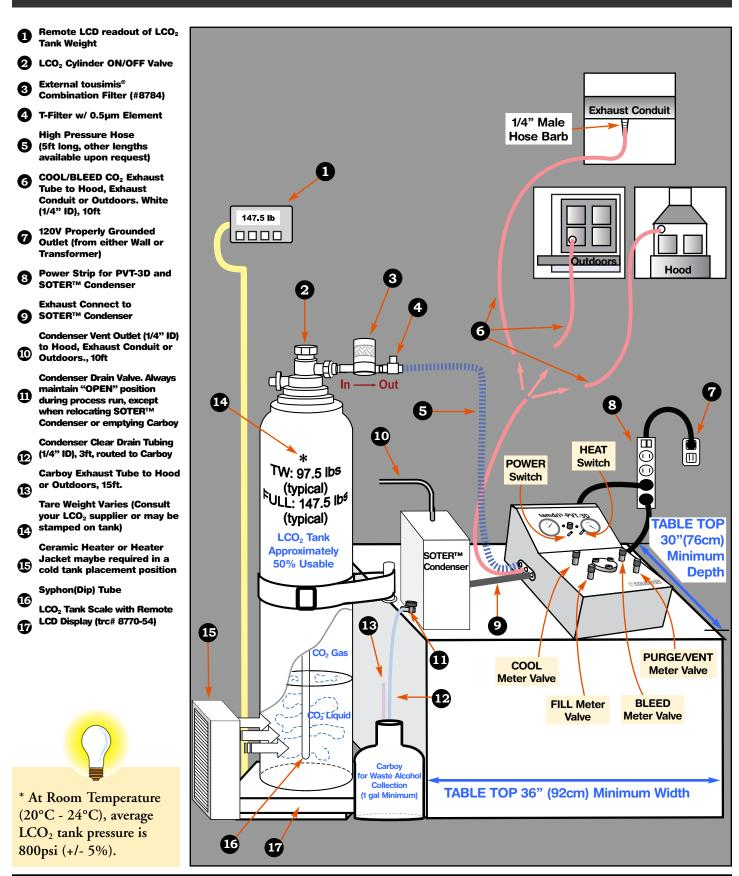
3. The tousimis<sup>®</sup> LCO<sub>2</sub> Filter Assembly (tousimis<sup>®</sup> catalog #8784) is factory installed directly onto the high pressure hose (See p.31-32). This helps prevent sample contamination from oil, water and particulates. Change the #8784A filter element with every 500lbs (226.8kg) LCO<sub>2</sub> tanks changes. The secondary 0.5µm T-Filter element may be removed, ultra-sonicated and reinstalled every 1 year.
