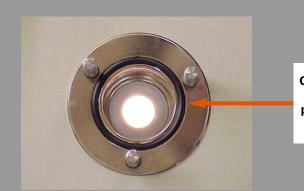
O-Ring (trc #8770-51) should be properly seated and dry prior to placing Chamber lid onto Process Chamber.
