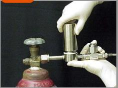
Hand tighten the housing body together firmly. O-Ring seats properly. Open main tank valve and check for leaks.
