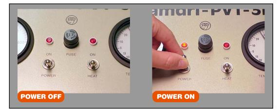
1. Turn power ON. Power light and chamber light will illuminate. Allow SAMDRI<sup>®</sup>-PVT-3D to warm up for 3 minutes prior to use. This allows time for the internal valve heaters to equilibriate.
