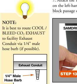
7. Attach the 10ft <u>White</u> exhaust tubing provided to the COOL/BLEED  $CO_2$  Exhaust outlet on the left-hand side of the SAMDRI<sup>®</sup>-PVT-3D. Tubing should be free of kinks which could block passage of rapidly exiting noisy gas or solid flakes of  $CO_2$ .
