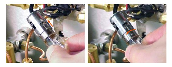
9. The Chamber Lamp is mounted into a "Bayonet" style lamp holder. Push Chamber Lamp towards the lamp housing and twist to the left to uninstall lamp (As shown below).
