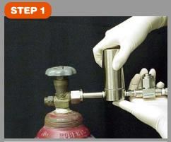
After all of the pressure is safely bled from high pressure line, unscrew Oil/Water Filter Housing by hand.
