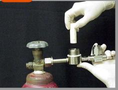
Position LCO<sub>2</sub> Filter Element (#8784A) into center of lower Oil/Water Filter Housing.
