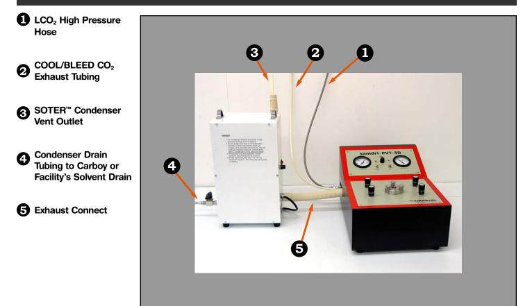
9. Connect Condenser Drain Tubing (clear) to a Carboy (1 gal minimum) or Facility's Solvent Drain. Condenser Drain Valve should always be maintained in the "OPEN" position during the process run, except when relocating Condenser or emptying Carboy. Connect Carboy Exhaust Tubing (white) to Fume Hood or Outdoors (See p.39 "Setup Overview").
