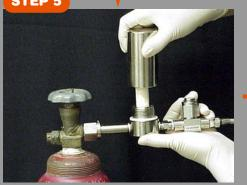
Carefully lower Oil/Water Filter Housing over replacement element (#8784A).
