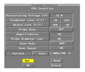
• When the column conditions are set, select **Preset Measurement**, and select all standards that are to be used and select **Acquire** to start the collection process.
