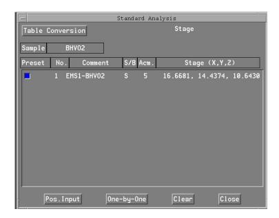
• From this screen, select "Pos. Input" to initialize the stage control panel which controls the points selected for analysis.
