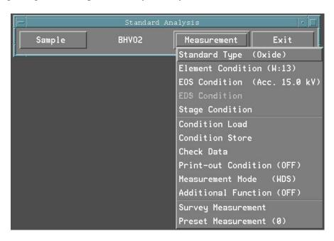
• First verify that the Standard type matches the type of analysis being performed, metal or oxide.
