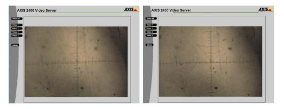
• The optical plain will show the flatness of the material being analyzed, if there is a flatness issue, it will be seen on the outer edges of the image and can affect the data if the crosshairs at the center cannot be focused.
